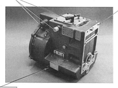
Connectors LOCTITE 577 pipe sealant
