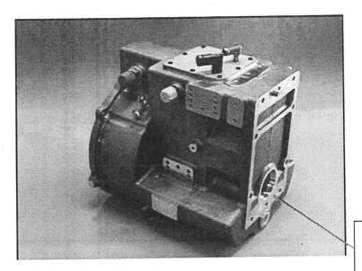
Gearbox/housing mating plane: LOCTITE 518 sealing compound
