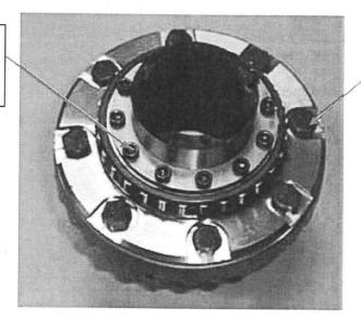
Crown bolt: 90N.m LOCTITE Blocpress 648
