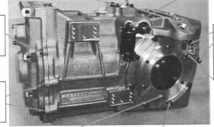
Push-pull lock bolt: 25N.m LOCTITE low-strength threadlock 222
