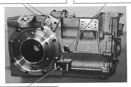
Reverse pin anti-rotation bolt: 22N.m LOCTITE sealant 577
