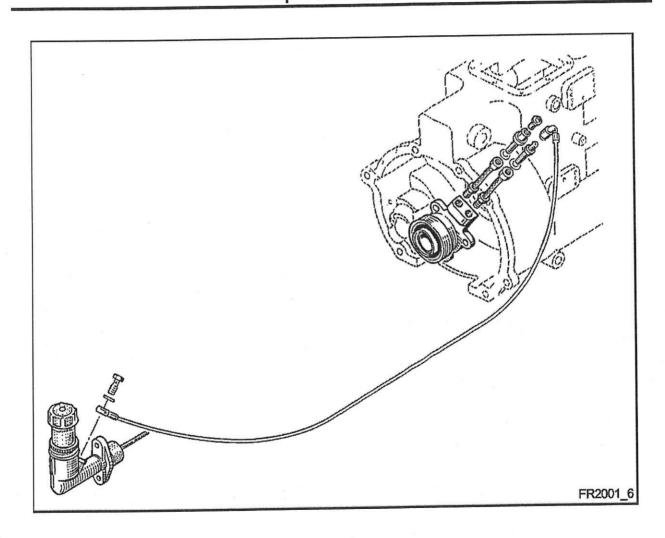
The clutch is dual-disc with hydraulic control (1), runs dry. It is installed on the front of the engine oil housing forming the clutch housing. It contains:
