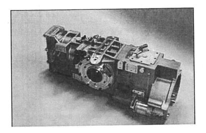
The Renault Sport gearbox is a SADEV SL75/14 FR 2.0, type it has 6 forward gears and one reverse which can quickly be changed.
