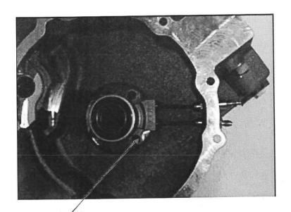
Hydraulic bearing bolt: 22N.m LOCTITE 243 medium-strength thread
