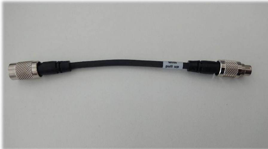
Fig. 1: F4 fuel pressure/temperature acquisition loom extension
