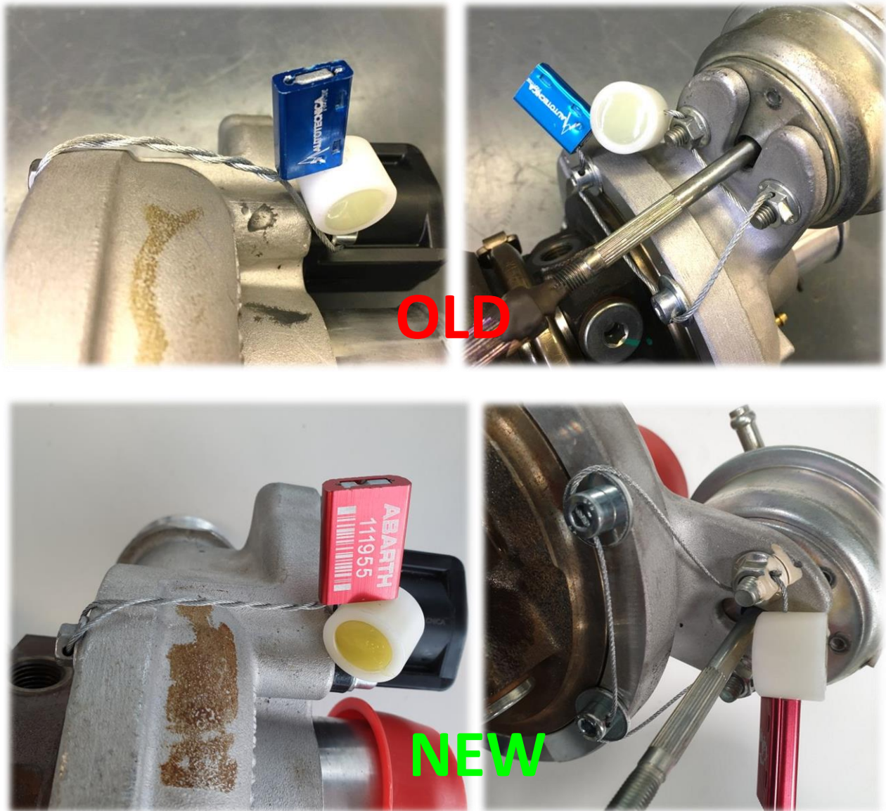
Fig. 2 : old BLUE and new RED + RFID sealed turbocharger
