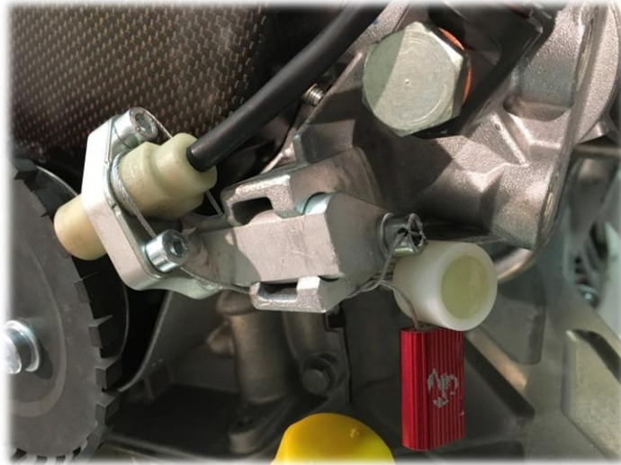
Fig. 3: RPM sensor bracket – RPM sensor, 2017 seal
